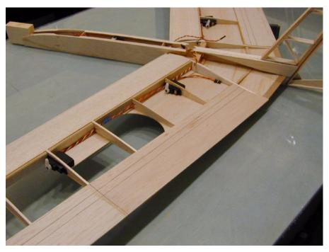
Our B 11 testbed under construction. The forward sweep angle, 18 degrees, matches the B 11 prototype. The root section is the CJ-25^2-09, the tip is the Clark X. The wing was built without twist. The wing servos drive outboard ailerons and inboard elevators, as on the original.
